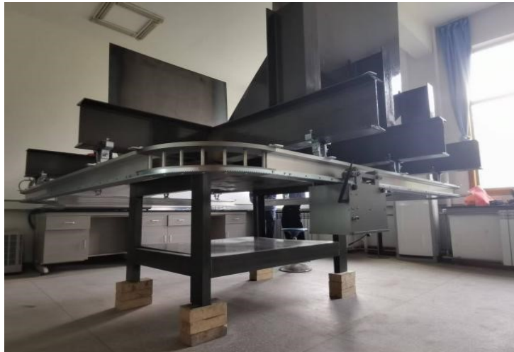
Figure 5. Simulation test platform for inspection robot operation.
